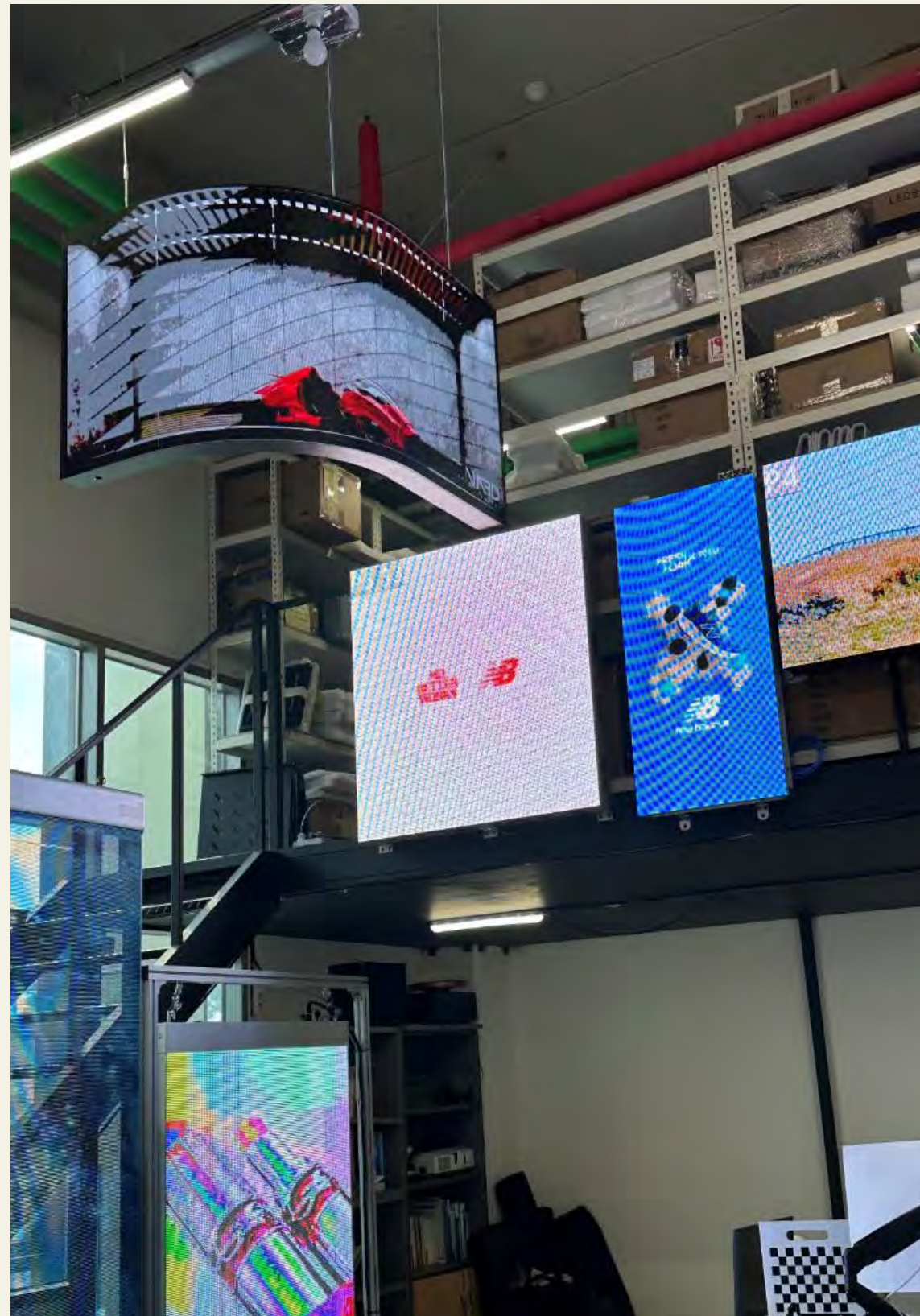
Flexible LED Steel Cabinet / P 2mm / 1,920x800mm
